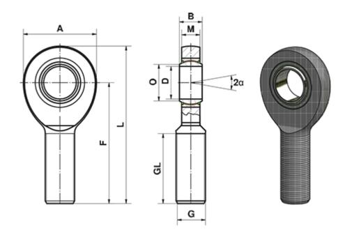
Α = 92 a (degrees) = 7 В = 28 D = 40 Dynamic load C (kN) = 277F = 150G = M39x3
